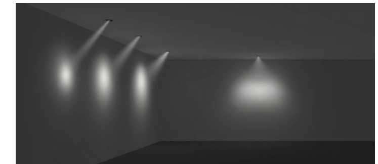
Emphasis of objects or architectural elements. Wide-beam illumination of larger objects or spatial zones.
