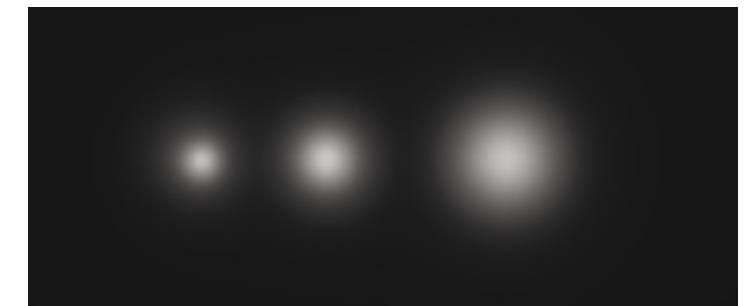
Emphasis of objects or architectural elements. Wide-beam illumination of larger objects or spatial zones.
